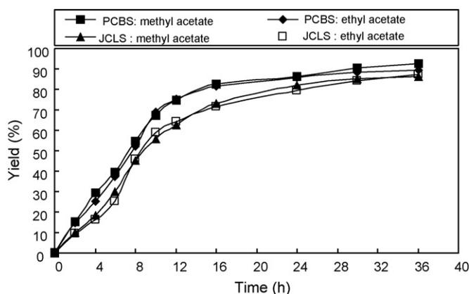
Fig. 3. Time course of ester formation during in situ reactive extraction. PCBS: *P. chinensis* Bunge seed, 4.26% of water content; JCLS: *J. curcas* L seed, 4.62% of water content. Five grams oilseeds, solvent/seed ratio of 7.5:1, 50 °C, 30% (w/w) of Novozym435 based on theoretical oil content, 180 rpm.
