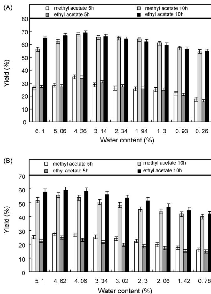
Fig. 2. Effect of water content of oilseeds on the ester yields: (A) *P. chinensis* Bunge seed; (B) *J. curcas* L seed. Reaction conditions: 5 g oilseeds, solvent/seed ratio of 7.5:1, 50 °C, 30% (w/w) of Novozym435 based on theoretical oil content, 180 rpm.
