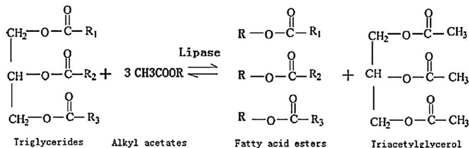
Scheme 1. Interesterification of triglycerides and alkyl acetates for fatty acid esters production.  $\text{R}_{1,2,3}$  represent long-chained fatty acids, R represents  $\text{CH}_3$  or  $\text{CH}_2\text{CH}_3$ .
