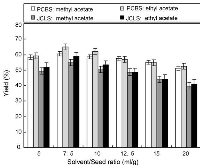
Fig. 1. Effect of solvent/seed ratio on the ester yields. PCBS: *Pistacia chinensis* Bunge seed; JCLS: *Jatropha curcas* L seed. Reaction conditions: 5 g oilseeds, 50 °C, 30% (w/w) of Novozym435 based on theoretical oil content, 10 h, 180 rpm.
